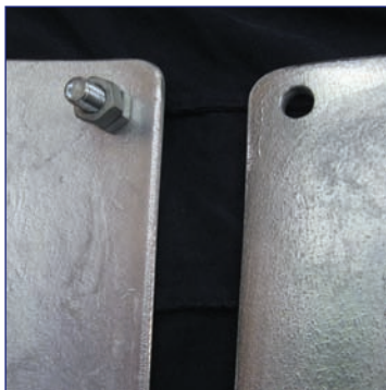
Do not balance a fan by drilling and grinding
