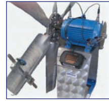
Fan pitching and two plane balancing
