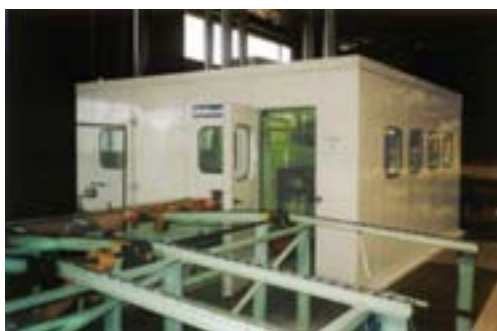
Acoustic enclosure in a timber processing factory
