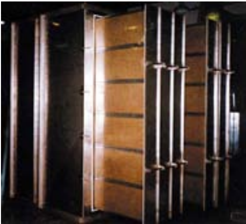
Removeable splitters allow for easy maintenance on this special design
